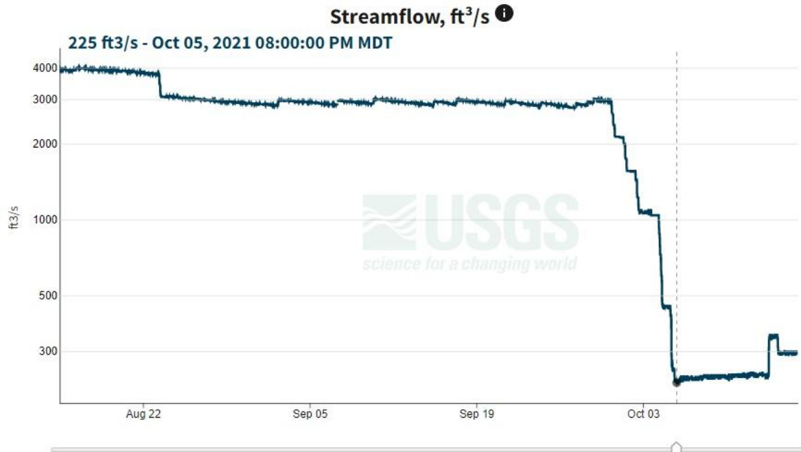
Figure 2. Release data showing abrupt ram-down of flows from Jackson Lake Dam between August 15 and October 15 in 2021.
